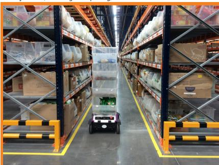
Autonomous Carts for Distribution Centers (ACDC®), a product of ALOG TECH, are autonomous mobile robots designed to operate safely within warehouses.
